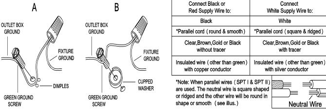
Twist wires together with plastic wire connectors until tightly joined, and wrap each connector with approved electrical tape. Be sure that no wire strands are exposed and then carefully tuck all wires into the outlet box.
