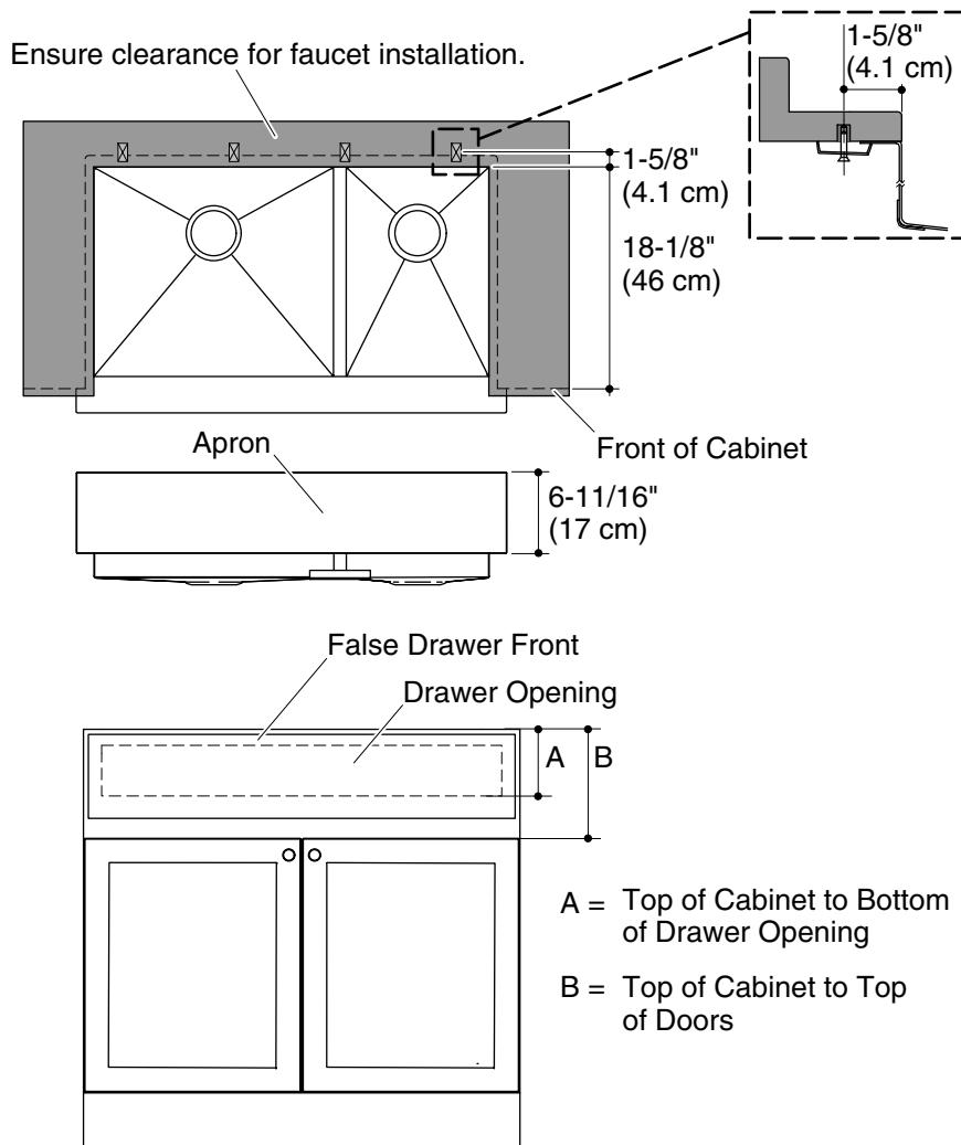
**IMPORTANT!** Before installing this sink, verify the opening height (A) is less than the apron height and the distance to the top of the doors (B) is greater than the apron height.
