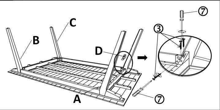
Attach the Wooden pad (D) to the table by using Short Screws ( $\Im$ ) and Screw driver ( $\Im$ ) as shown in picture below.
