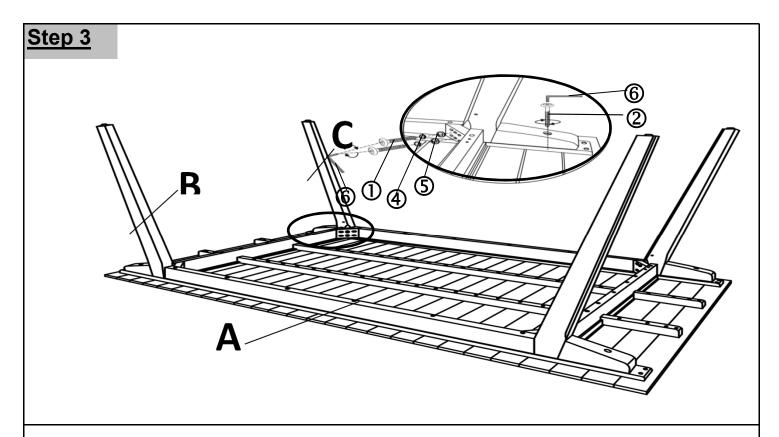
Attach Second Leg (C) to Table Top (A) as shown in picture above.
