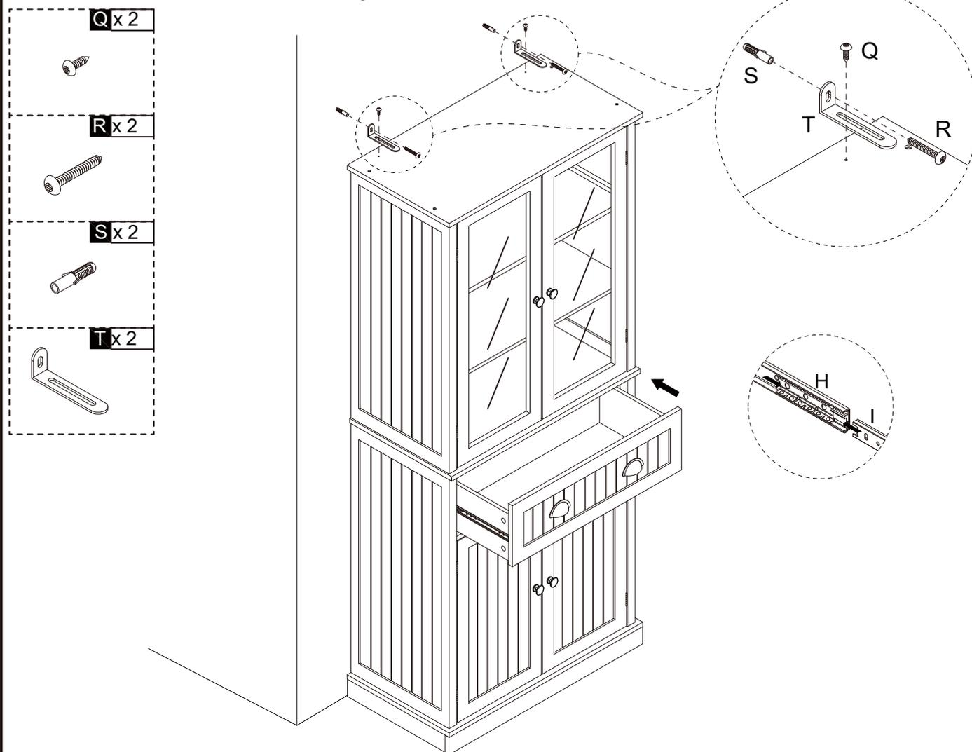
**EN** If it is a solid wall, please use expansion and self-tapping screws, if it is a wooden wall, only use self-tapping screws, please do not overtighten the screws
