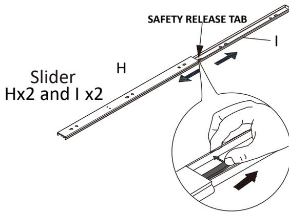
H and I are shipped together to maintain the oil for the ball bearings. Note that you need to tip up the safety release tab to take out the I part prior to assembly.
