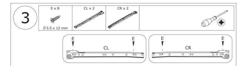
Fix rail(CL) and (CR) to panel 9 with screw(E) as shown.
