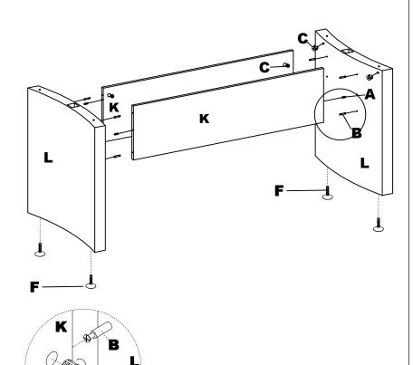
NOTE: The arrow on the face of the Cam (C) should point towards the Cam Post (B) for proper alignment.
