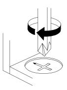
Turn cam lock clockwise to tighten.
