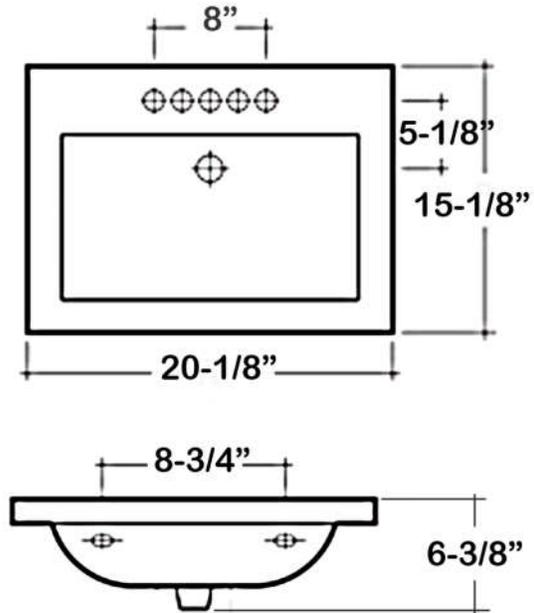
Dimensions of fixture are nominal and may vary within the range of tolerances established by ASME Standard A112.19.2-2013. Dimensions and specifications subject to change without notice.
