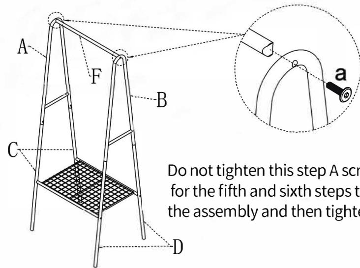
Do not tighten this step A screw, wait for the fifth and sixth steps to complete the assembly and then tighten.
