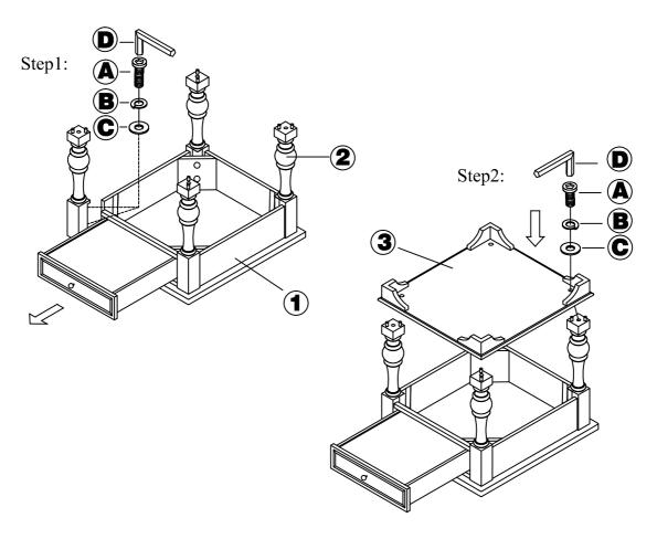
NOTE: DO NOT TIGHTEN ALL THE BOLTS UNTIL THEY ARE INSTALLED IN CORRESPONDING HOLES!
