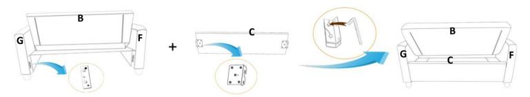
Step 4: Install 4 wheels on bottom of trundle bed, please use tools to set screws .
