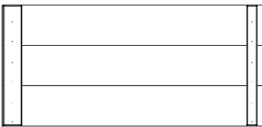
RP2 | LEFT PORCH ROOF PANEL - W2A02651 (1) 1\frac{5}{8}" \times 15\frac{5}{8}" \times 32\frac{7}{8}" (42x396x834)
