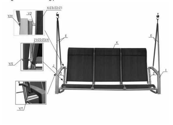
IV)Attach completed swing section to the main frame using the springs provided, parts M
