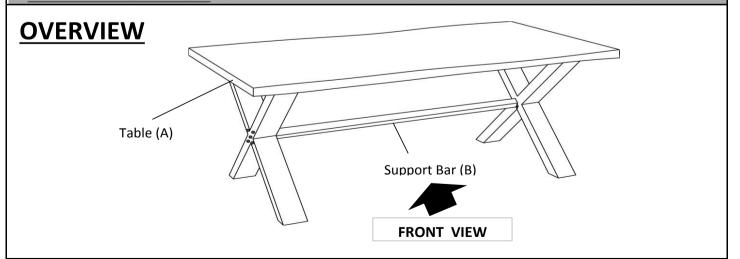
This <u>Table</u> has multiple parts and may require up to some 15 minutes to assemble. To give you an overview of the <u>Table</u> parts, the above picture is to help you put the various parts into perspective. Please read through the instructions here below to familiarise the parts and steps before assembly.
