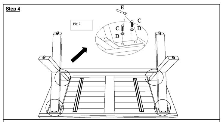
Secure Legs to Table by using Bolts (C) and Flat Washers (D) with Spanner Wrench(E) as shown in Pic.2 above, at all 8 positions.
