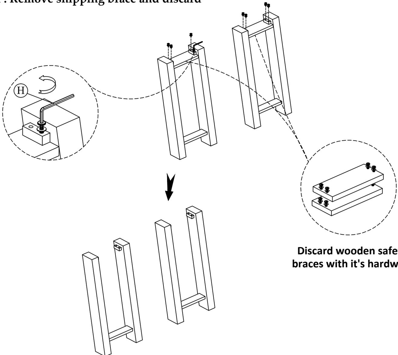
**Step 2 : Do not fully tighten the bolts**
