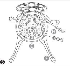
Repeat Steps 4 and 5 to assemble second chair. Adjust the pre-installed Rubber Feet ① until the Bistro Set sits level on the ground. Check ALL Nuts on table and chairs for tightness and adjust as necessary using Wrench ③. Lastly, cover all Nuts with Plastic Caps ①/①.
