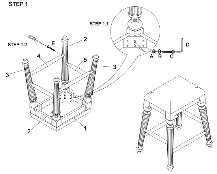
Do not fully tighten all screws and bolts until the entire item is completely assembled.
