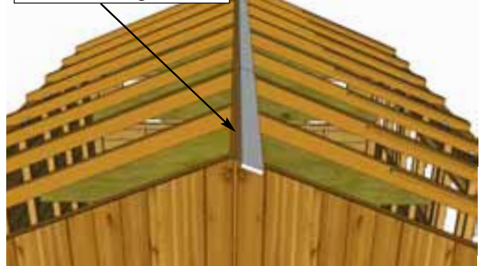
Flush to Ridge Board
