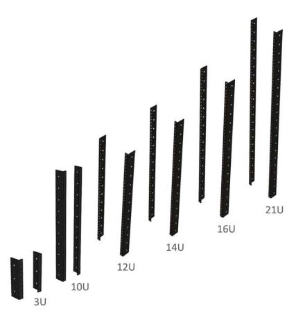
**RR Series** rack rails are available in various capacities - **RR3**, **RR10**, **RR12**, **RR14**, **RR16** and **RR21**. EIA compliant racks in 3-21 rack units. Standard side to side spacing for these rack rails is 19.125".
