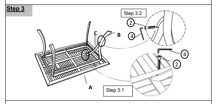
Place Leg Support(C) between Table Top(A) and Leg(B), as shown above. **3.1)** Secure Leg Support(C) to Table Top(A) using Screw(2) with Allen
