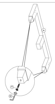
with Allen Key (H) provided. Then attach each Slat (7) to Side Rail (6) using 1 Wood Screw (F). Attach each Support Leg (8) to each Slat (7) using Allen Bolts (B). Tighten all bolts
