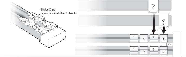
3 Adjust the panel track to the width needed. Be careful not to over extend the track and cause it to separate completely.
