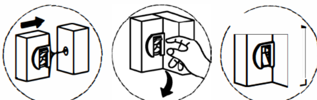
Tab in opened position Pull tab down to lock Tab in locked position
