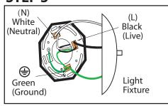
Connect (push) electrical wires from fixture into correct inserts. Black (live), White (neutral), Green (ground)
