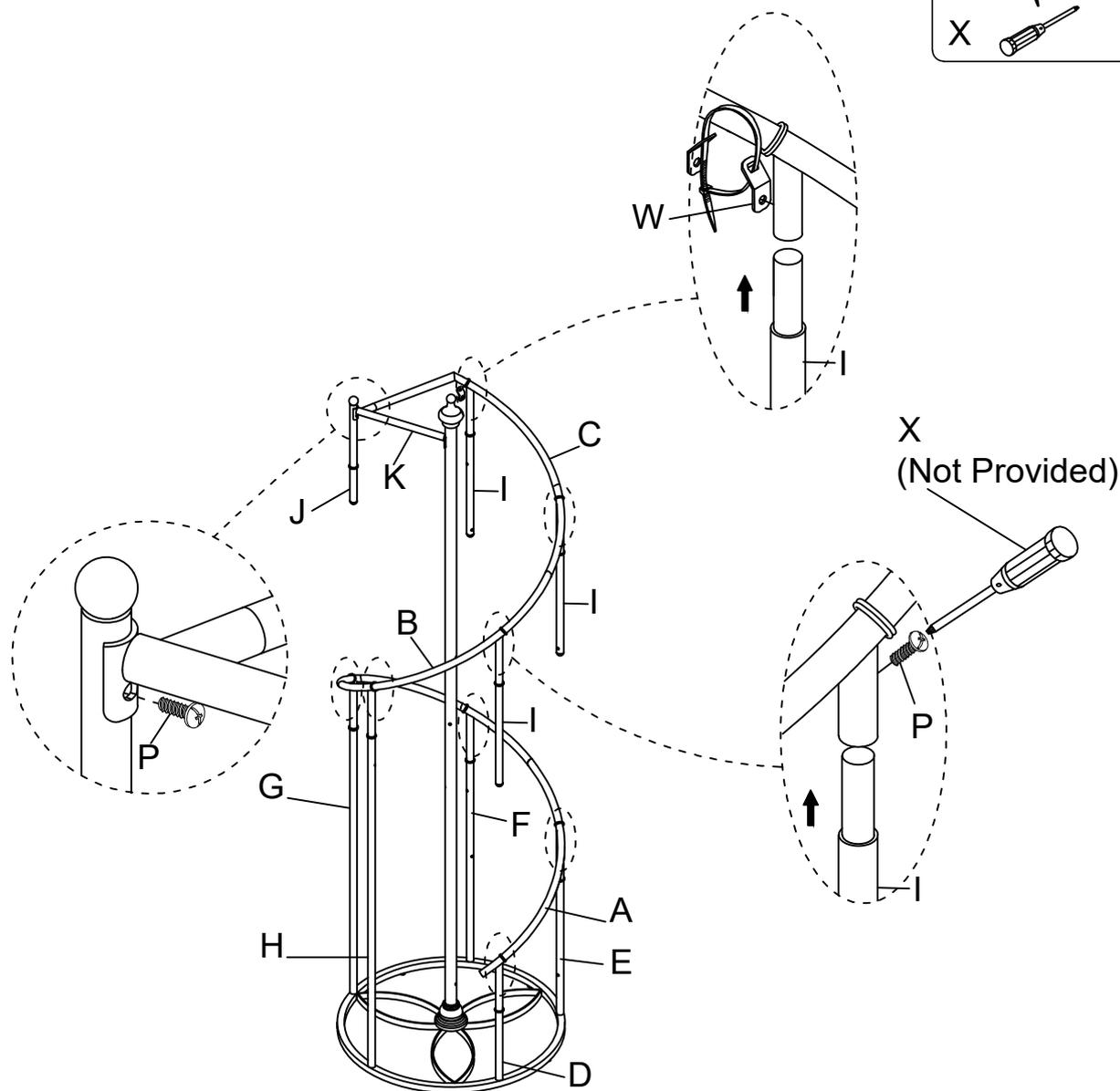
**6** Assemble Shelf Frame (N) to Center Post (L), Top Post (J), Upper Post (I), Bottom Post (H), Bottom Post (G), Bottom Post (F), Bottom Post (E) & Bottom Post (D) from top to bottom, then using Bolt (P) to fasten by Screwdriver (X).
