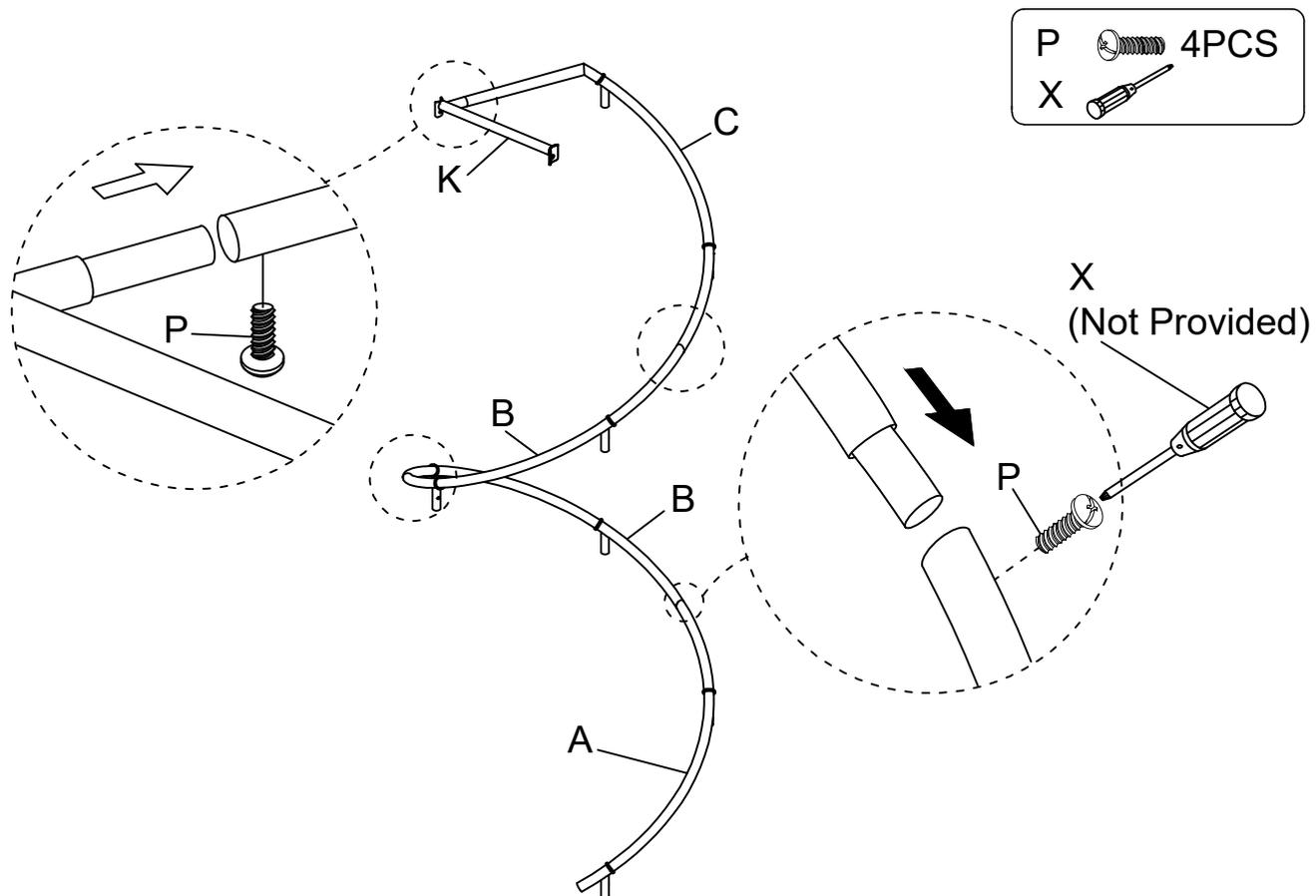
**4** Assemble Connector Bar (K) to the Center Post (L) with Bolt (P), then fasten by Screwdriver (X).
