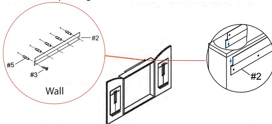
Step 2: Select a drill bit that is roughly the same diameter as the **Plastic Anchors (#5)** included in the hardware pack. Once holes have been drilled, use a hammer and tap the **Plastic Anchors (#5)** into the holes. After the anchors are secure, attach the **Hanging Plate (#6)** using **2" Screws (#3)**.
