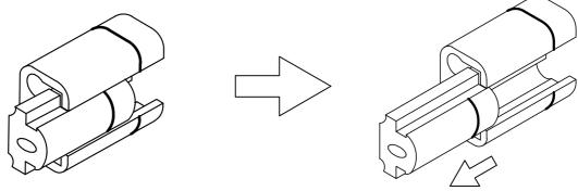
You can pull the buckle out by following the direction indicated by the arrow
