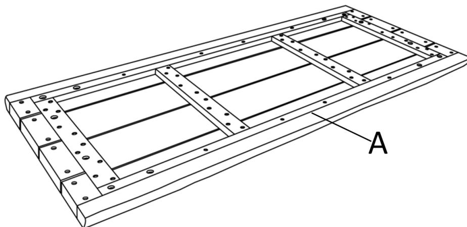
With the assistance of an adult, lay the Table top (A) facedown onto a clean, flat surface to avoid any scratches or damage to the product.
