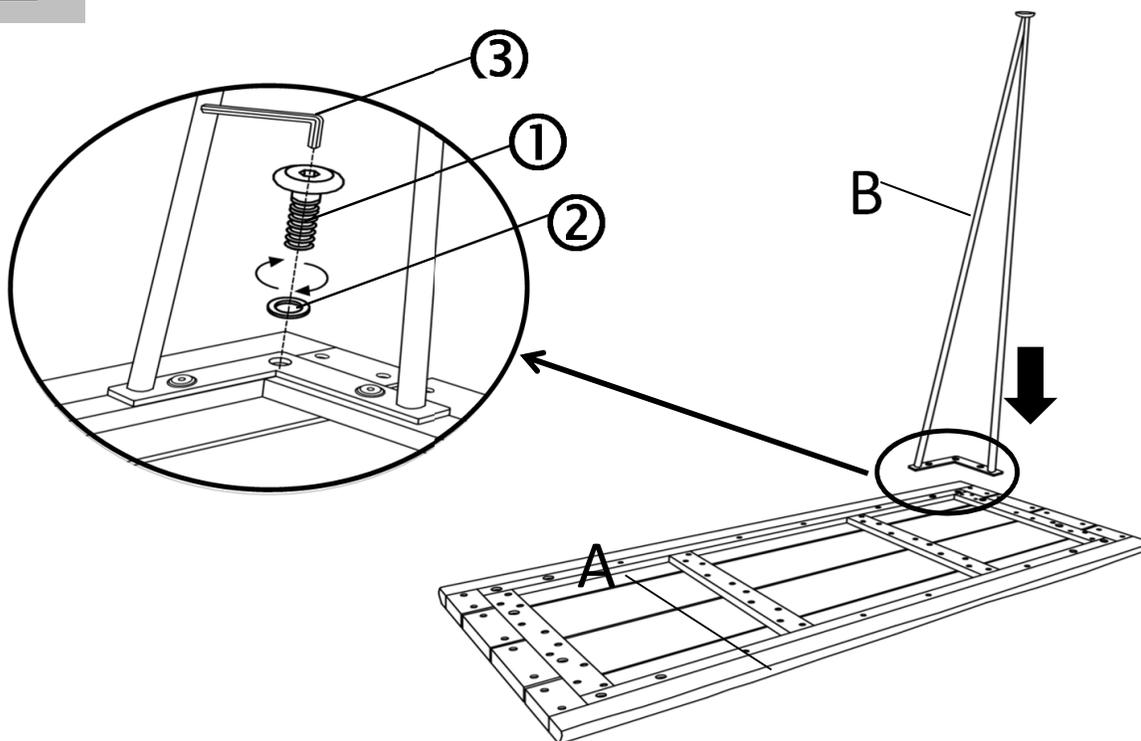
Insert **one of legs** (B) into the table top (A), put the flat washer (②) and bolt (①) as above picture.
