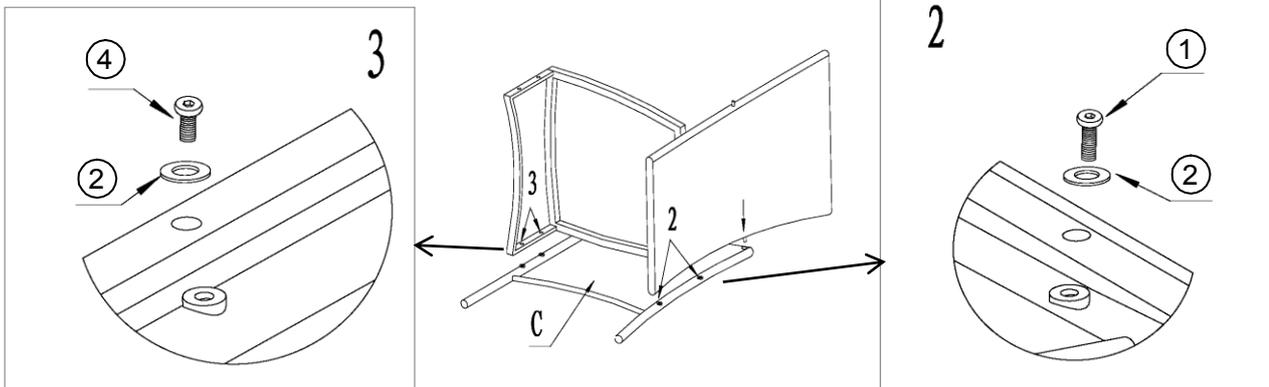
Place the Left Armrest/Leg(C), as picture above so as to be attached to the Backrest (A) and Seat(B) using Hardware(①, ④, ②) with Allen Key(③).
