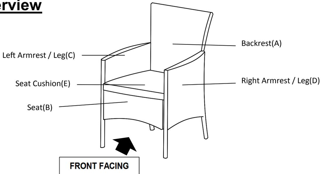
This Chair has multiple parts and may require up to some 30 minutes to assemble. To give you an overview of the Chair parts, the above picture is to help you put the various parts into perspective. Please read through the instructions herebelow to familiarise yourself with the parts and steps before assembly.
