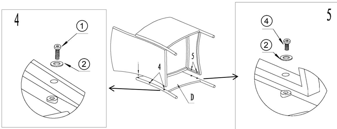
Place the Right Armrest/Leg (D) as pictured above and affix to Backrest (A) and Seat(B) using Hardware(①, ④, ②) with Allen Key(③) as shown in Picture 4 and Picture 5.
