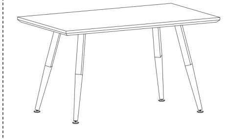
**STEP 1:**:Place the top A upside down on clean padded surface. turn all the legs B outward, use bolt 1, flat washer 2 and spring washer 3, allen key 5 to connect the legs B with top A, place foot 4 on bottom of the legs B, make sure all holes aligned and fasten all bolts to secure.
