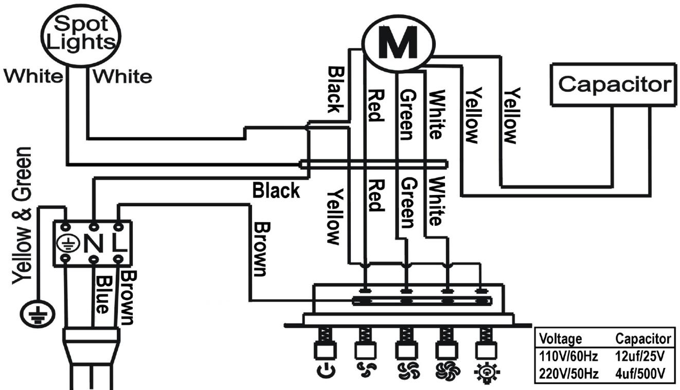
NOTE: Wiring Diagram shown above with GU10 light configuration. A transformer is required for MR16/J4 Lights.
