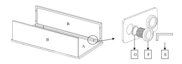
$Step\ 2.$  Attach End Panels (C) to Side Panels (B) using Bolts (F), Washers (G), Brackets (H) & Allen Key (E).
