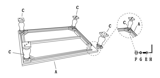
Attache bottom(B) to leg(C) by using screw(D), flat washer(F), spring washer(G) and allen wrench (H) as shown.
