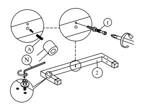
Step 24: Secure the frame using hardware parts C, F, N and O with a screwdriver (not provided).
