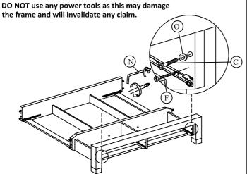
Step 23 : Attach the footend (2) to the frame (24) using the screws and hardware part I , J , K and N  $\,$
