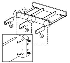
Step 19 : Secure the frame using hardware parts  $\boldsymbol{B}$  and  $\boldsymbol{N}$  .
