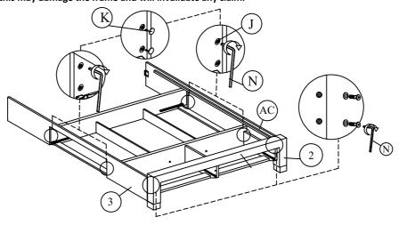
Step 28: Loosen the pre-inserted screws on the headboard (1) using hardware part  $\mbox{\it N}.$
