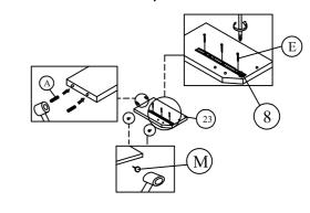
Step 15 :Attach the drawer runner from pack 2 (8) to the drawer center divider (24) using hardware part E and screwdriver(not provided).Insert hardware parts A and M to the drawer center divider (24) using a small mallet (not provided). the flip drawer runner from pack 2 (8) to the other side and repeat the same step.
