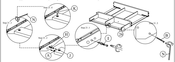
Step 22: Insert hardware part A to the footend (2) using a small mallet (not provided), then insert hardware part I using a screwdriver (not provided).
