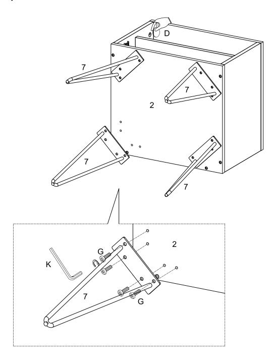
Using bolt (G) secure part (7) to part (20 with hex key (K) ,then using sticker (D) cover the hole as per diagram.
