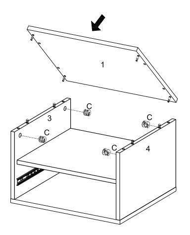
Using cam lock (C) secure part (1) to parts (3,4) as per diagram.
