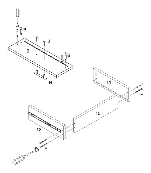
Using screw (F) secure parts (11,12) to part (10), using bolt (J) secure handle to part (9), and using cam bolt (B) secure part (9) with Philips head screw driver as per diagram.
