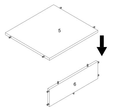
Attach part (5) to part (6) as per diagram.
