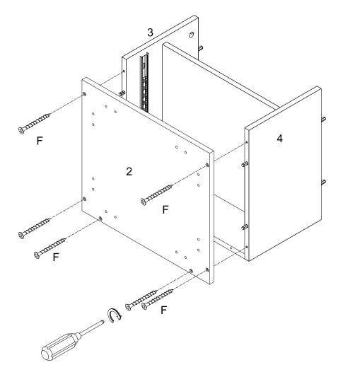
Using screw (F) secure part (2) to parts (3,4) .
