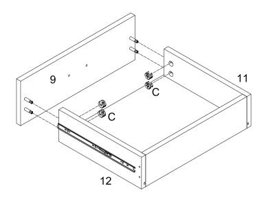
Put part (8) to parts (10,11,12), then attach part (9) to parts (11,12) as per diagram.
