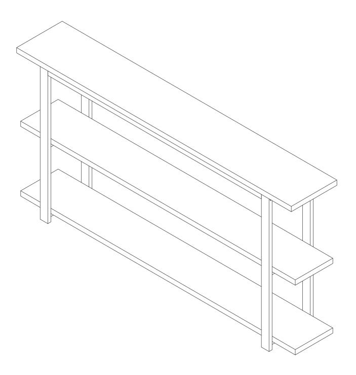
**Notes:** Don't tighten screws completely at first, just in case parts were assembled wrong and need disassenbled. Tighten screws at last when all parts are put together.
