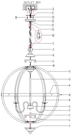
Step A1: Slip stem (O) over the wires and then thread it into the top of fixture loop (S). Slip Fixture body (M) over wires and then thread it onto the top of stem (O).
