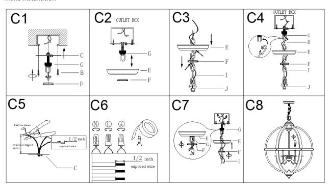
Step C1: Remove the threaded ring (F) from collar loop(G). Attach the single bar (C) to outlet box with mounting screws (B). The side of single bar marked "GND" must face out, Unscrew the collar ring (H) from the collar loop.
