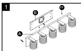
1.Remove four mounting screws (FF) to separate the mounting bracket(B)from back plate(A).
