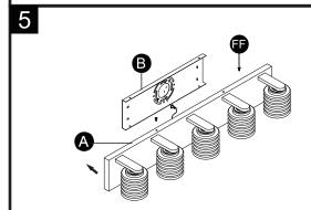
5. Attach the back plate(A) to the mounting bracket(B), and then secure it with mounting screws (FF).
