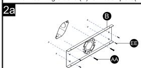
2.Fix the mounting bracket(B) to the wall.
