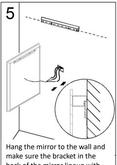
back of the mirror lineup with the mounting bracket properly.
