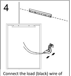
the Dimming driver cable (white) to wall switch if used, otherwise to a common hot wire. Connect the load (black) wire of the Touch Switch cable (black) to hot wire.
