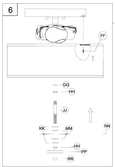
6. Attach shade (B) to fixture (A) using the 3 screws (FF). Then attach the glass diffuser using the hardware shown below, making sure to follow the order shown below to attach safely.
