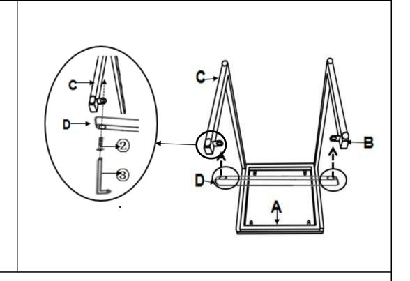
Attach the Base Support Bar(C) to Side Panel(B) and Side Panel(C) using Bolts(2) with Allen Key(3).
