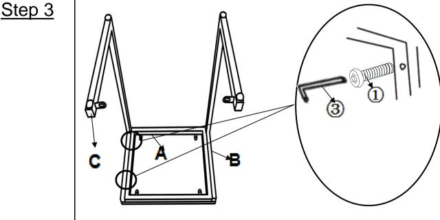
Attach the Side Panel(C) to Top Panel(A) using Bolts(1) with Allen Key(3) as shown above.
