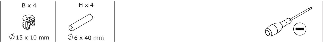
Attach plate 8 to plate 13,14 with wooden dowel(H) and turn cam locks(B) clockwise to tighten as shown.
