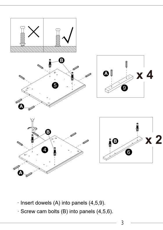
•The provided glue(H) is to secure When first inserting dowels, locate the wood dowels(A) in place. appropriate hole for the dowel , place a small amount of glue in the hole and insert the dowel.
