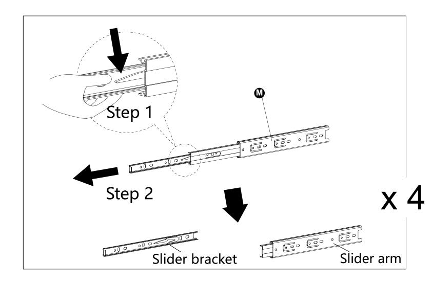
$\cdot$  Separate the slide bracket from the slide arm as per diagram.
