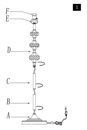
Step 1 Make sure all parts could be aligned before assemble Do not rotate lamp body too hard avoid base screm broken Pull cord through lamp base(A) to tighten stem connections, make sure the screw nut at the bottom of the lamp is tightened Insert the bulb(H) into the socket(F).
