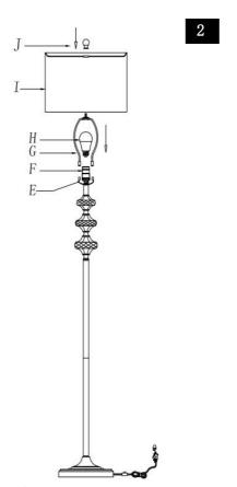
Step2 Insert the Harp (G) into the Saddle (E). Put the shade(I) on the Harp(G),then tighten the Finial (J)into the Harp (G)
