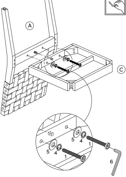
Righty-tighty! Secure the Seat Frame (C) to the Chair Back Assembly (A) using the two sets of Flat Washers (5), Lock Washers (4), and ¼ x 3½ inch Hex Button Head Bolts (3) in the holes pictured below.
