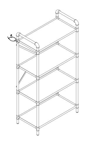
Do not tighten screws until completely assembled.
