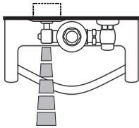
2. As the user enters the beam's effective range (15" to 30") the beam is reflected into the OPTIMA Scanner Window and transformed into a low voltage electrical circuit. Once activated, the Output Circuit continues in a "hold" mode for as long as the user remains within the effective range of the Sensor.
