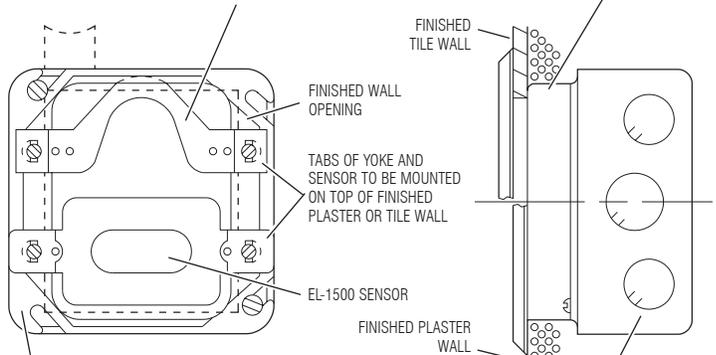
NOTE: INSTALL PLASTER RING SO THAT SCREW HOLES ARE ON THE LEFT AND RIGHT SIDE OF BOX (VIEW WITH COVER REMOVED)
