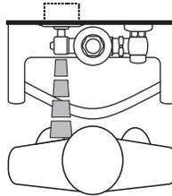
3. When the user steps away from the OPTIMA Sensor, the circuit immediately initiates an electrical "one-time" signal that operates the Solenoid. This initiates the flushing cycle to flush the fixture. The Circuit then automatically resets and is ready for the next user.
