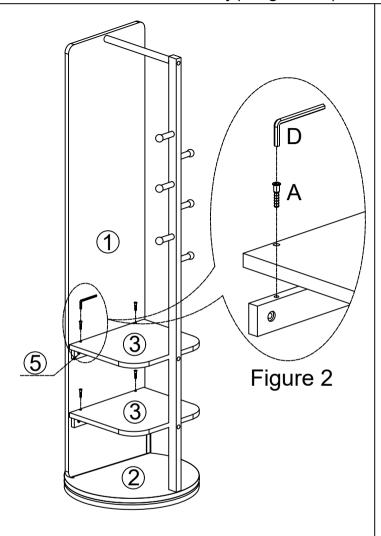
Assemble part 3 on top of part 5 with hardware A/D as in figure 2.
