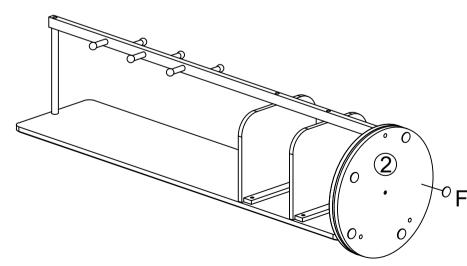
Assemble as shown, attaching accessory F to the bottom of the base.
