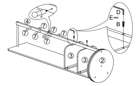
Assemble as shown, first lay part 3 flat to the designated position, align the holes on the end face of part 3 with hardware B/D, and then cover the holes with hardware E.
