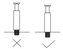
Below shows how the pins are used to assemble the panels together.
