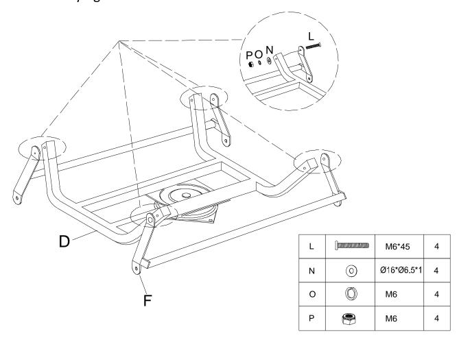
**Step 7**: Attach swivel plate to part G with 4pcs bolts J, 8pcs washers N, 4pcs spring washers O, and 4pcs nuts P, using Allen wrench S and wrench T. Note: Don't fully tighten the bolts.
