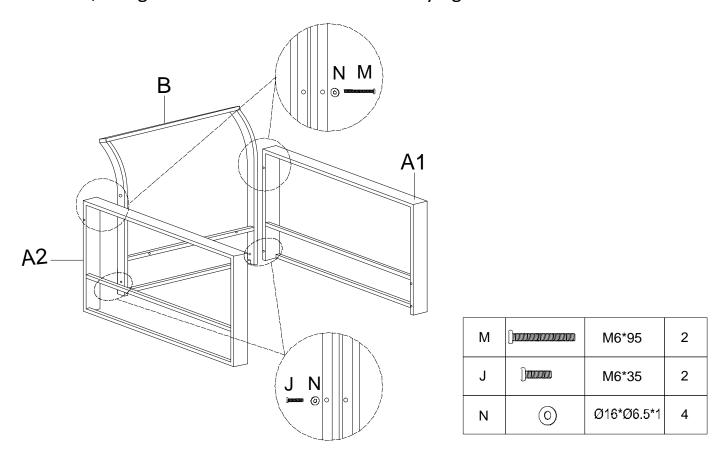
**Step 2**: Attach seat C to arms A1 & A2 with 4pcs bolts J and 4pcs washers N, using Allen wrench R. Note: Don't fully tighten the bolts.
