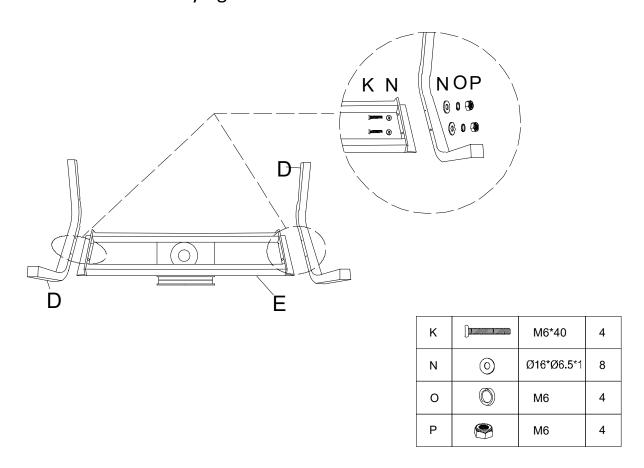
**Step 5**: From vertical direction, attach 2pcs part D to part E with 4pcs bolts K, 8pcs washers N, 4pcs spring washers O, and 4pcs nuts P, using Allen wrench S and wrench T. Note: Don't fully tighten the bolts.
