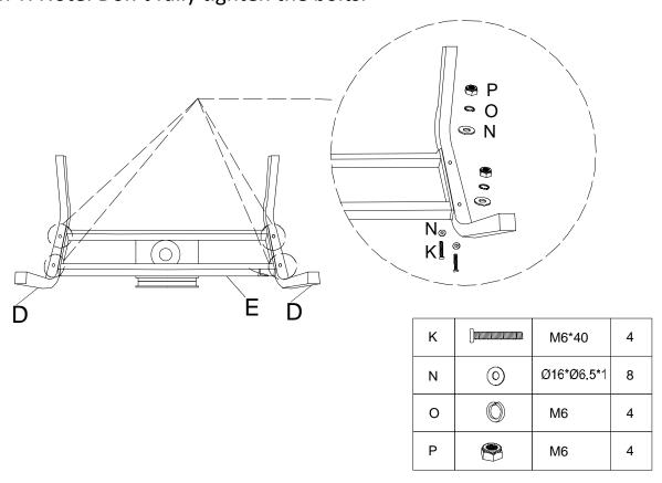
**Step 6**: Attach 2pcs part F to part D with 4pcs bolts L, 4pcs washers N, 4pcs spring washers O, and 4pcs nuts P, using Allen wrench S and wrench T. Note: Don't fully tighten the bolts.
